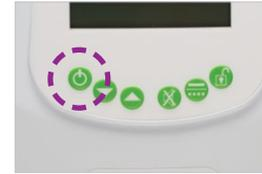
To change the canister make sure the pump is powered off (if still running, press and hold the UNLOCK button, followed by the RUN/STOP (Power) button).
