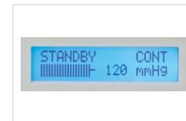
Power on the pump by pressing the RUN/STOP (Power) button. The pump is now in STANDBY mode. Ensure the pressure is set to the prescribed level by pushing the up or down arrows.
