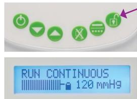
After 1 minute in RUN mode, the locked key function is activated. This is shown with a padlock sign.
