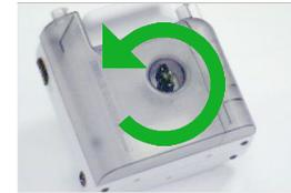
Rotate the locking knob 1/4, turn counter-clockwise and remove the canister. Dispose of the used canister according to local clinical waste policy.
