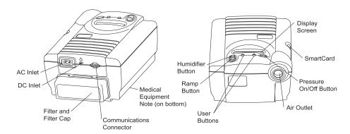
**AC Inlet** ...... Connect the power cord here.
