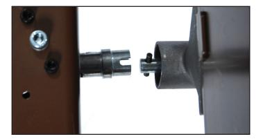
• Make sure the slot on the spring loaded shaft engages the roll pin on the gear box.
