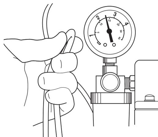
*Step 5: Check for proper negative pressure*
