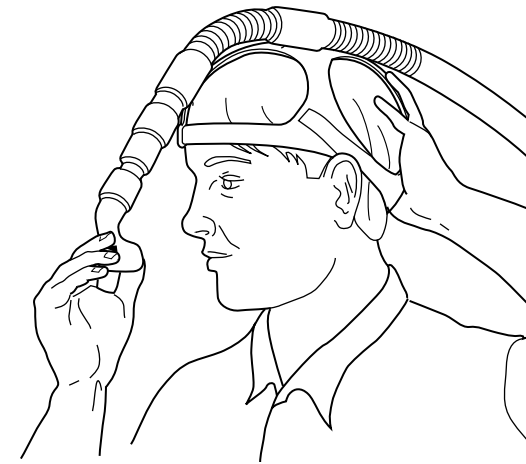
Adjusting the headgear assembly
